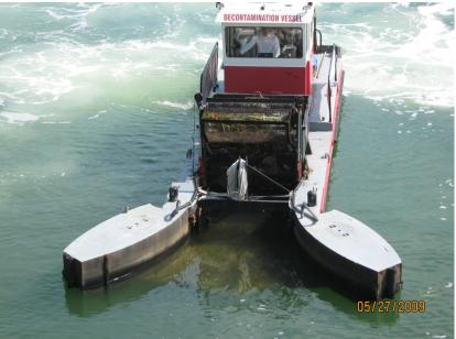
The trash recovery system is removed and this oil recovery system is inserted inside the Scavenger2000.
